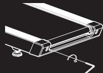
IF THE RUNNING BELT MOVES TO THE LEFT, TURN THE BOLTS ON THE LEFT SIDE  $\frac{1}{4}$  TURN CLOCKWISE, THEN TURN THE RIGHT BOLT  $\frac{1}{4}$  TURN COUNTER-CLOCKWISE. IF THE BELT DOES NOT MOVE, REPEAT UNTIL IT CENTRES.
